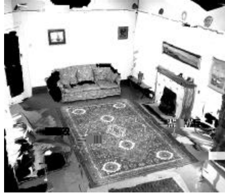
Figure 8: 3D wire-frame model generated from 3D data captured by a laser range finder (left), and for
